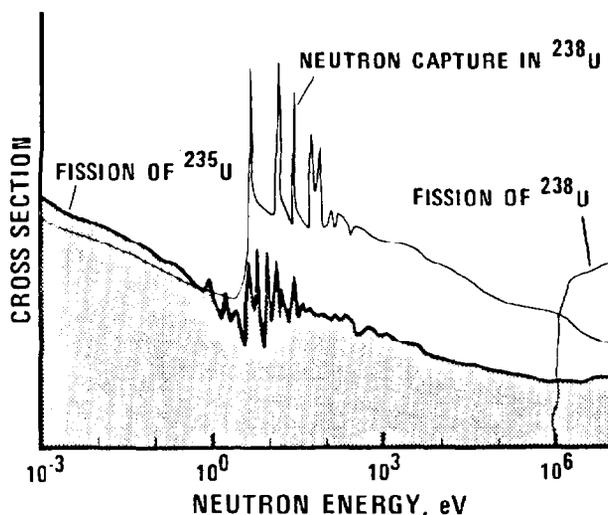
FIG. 3.6: Energy dependence of the fission and capture cross section in uranium.
