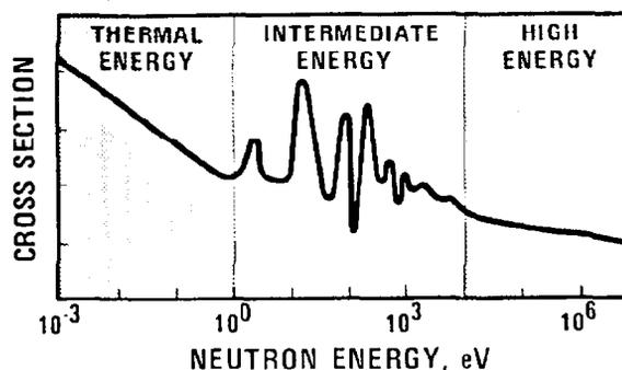
FIG. 3.7: Typical energy dependence of neutron capture cross sections for many nuclei.
