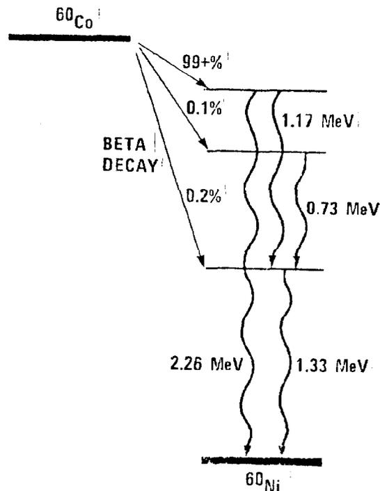
FIG. 3.1: Decay processes for Cobalt-60 and energy levels of Nickel-60.
